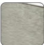
22 Edelstahl matt geschlichtet stainless steel turned finish
